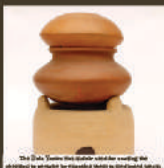
Purna Yantra was an apparatus used for sublimation and distillation.
